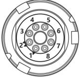
View from solder connector side of the connector
