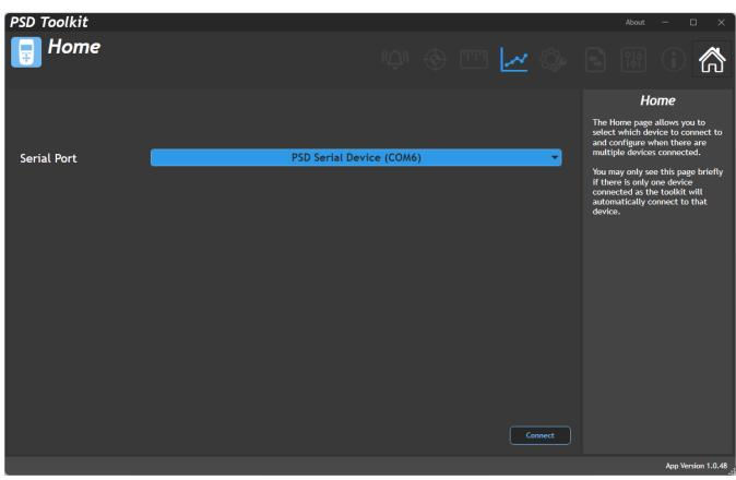
When you connect the handheld to the PC using a USB cable it creates a virtual COM port on the PC. All detected TRX devices are displayed in the drop-down list and you need to select the appropriate one. If only one handheld is detected you may not see this page as the Toolkit will automatically select and connect to it.
