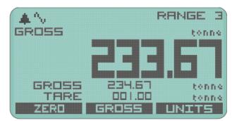
The Gross value and value of Tare are continuously displayed under the main value. Soft keys allow you to Zero the main display, switch back to full Gross value or change displayed units.
