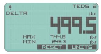
Soft keys allow to Reset the min and max to the current value. i.e. zero the Delta. The usual Units selection is also available.
